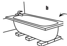
Now position your bath in place with the side and back situated on the brackets. Check again with the spirit level if the bath is still level on all sides.
