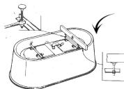
**C**. Turn the bath upside down on a carpet or non scratch surface. Use straight edge and spirit level to set feet 3mm above flange.
