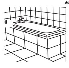
Plaster walls and tile where wanted and or needed. Use **only** a mildew resistant silicone sealant between where the tiles and bath come together.
